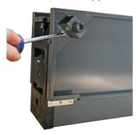
2. Fix the Media Hanging Base Bracket to each side of the machine using the four self tapping screws supplied - (ensure the diagonal countersunk holes face inwards on the machine)
